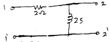
(b) Find the Current i(t) in the following Circuit Using Laplace Transformations Switch closed at t=0, Assume all the initial conditions are zero.
