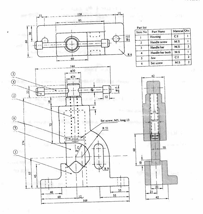
Fig. 1.0 Assembly Drawing of Pipe vice
