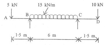
13. Determine slope and deflection at D and C for the overhanging beam shown below: 10
