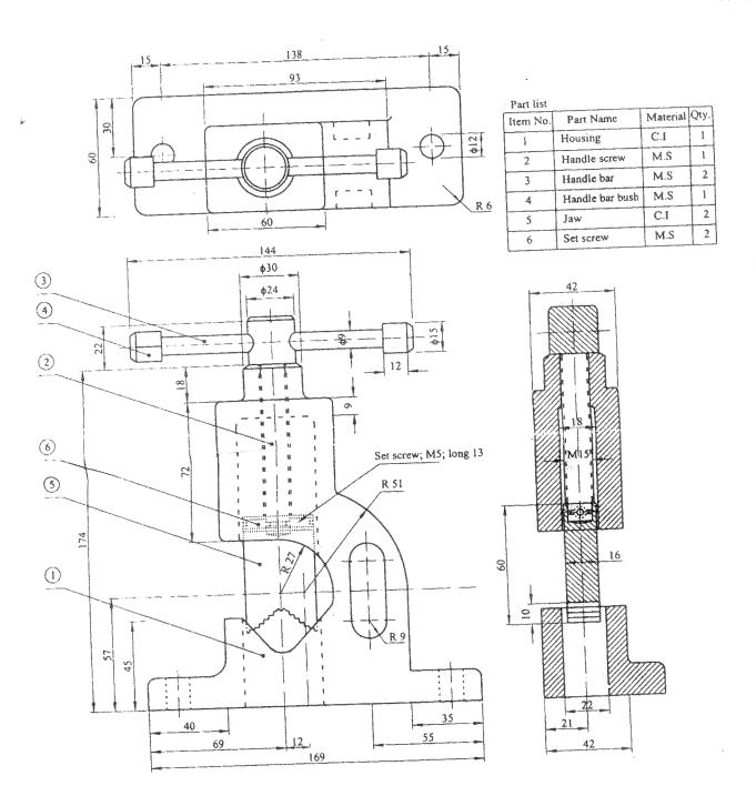
Fig. 1.0 Assembly Drawing of Pipe vice
